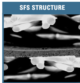
Cross-section of BLOCK-IT* 380 spunbond/film/spunbond laminate.
